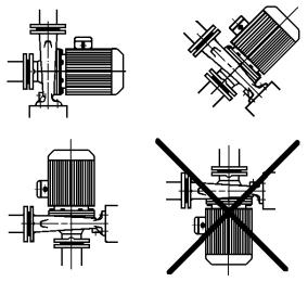
It is possible for the pump/motor assembly to be supported by the connecting pipework if it is suitably stable and rigid. For hot, damp environments, the preferred orientation is horizontal.
