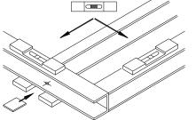
Level with shims between baseplate and packing pieces.
