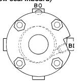
BO - Rp ¼ in. barrier liquid outlet BI - Rp ¼ in. barrier liquid inlet
